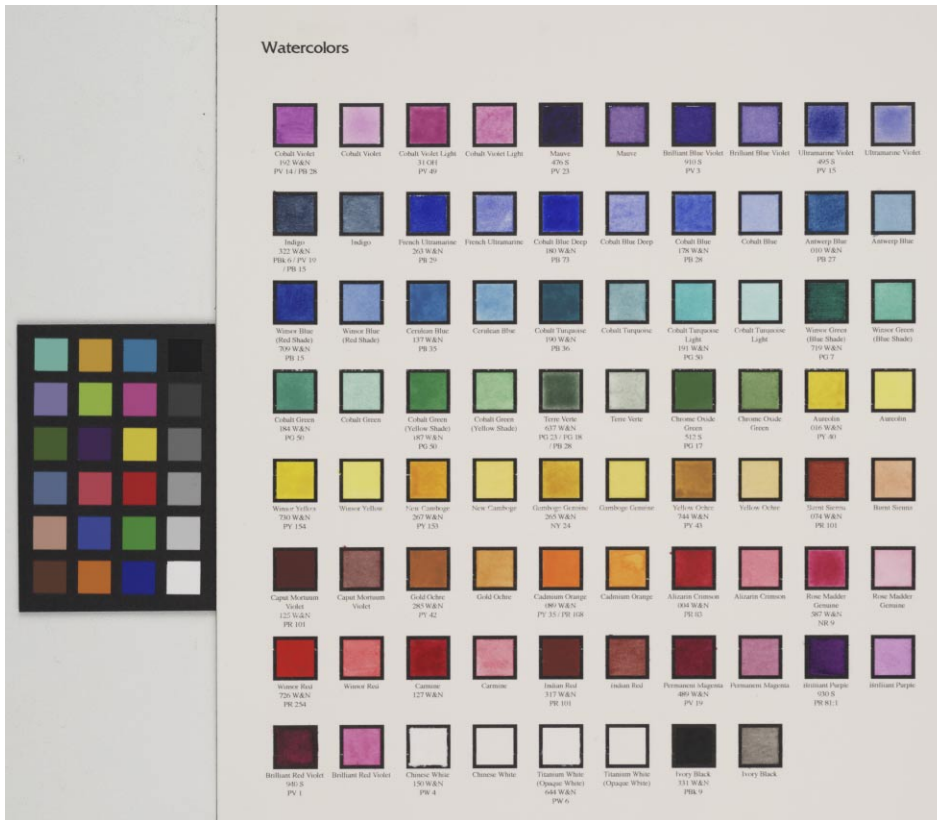
Figure 16. Watercolor test patches photographed with a Better Light Super 6k camera under fluorescent illumination and equipped with two filters.
